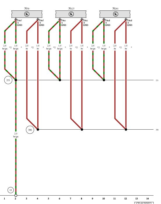
Ignition coil 1 with output stage, Ignition coil 2 with output stage, Ignition coil 3 with output stage
